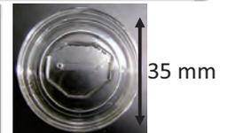
We designed the PDMS-based microfluidic channel for the LbL method in the channel, and formed an inlet center region that was parallel to the flow direction from the inlet to the outlet
