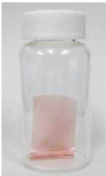
**Figure 1.** Photoelectric dye-coupled polyethylene film (**OUREP<sup>TM</sup>**): a novel type of retinal prosthesis.
